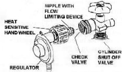
**The LP Gas Cylinder is not included with the Gas Grill.** Be sure to purchase one with the QCC valve. This valve is recognized by the external threads on the inlet port of the valve. QCC equipped cylinders are available from your gas grill dealer. **Any attempt to connect the regulator, by use of adapters or any other means, to any other valve could result in damage or fire, and may negate the important safety features designed into the QCC-1 system.**
