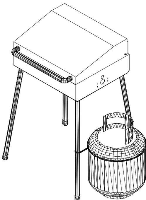
Secure the Propane Tank by securely latching the Support Ring Latch. (as shown).
