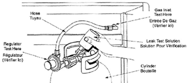
4. Leak test the connection. See "leak test".
