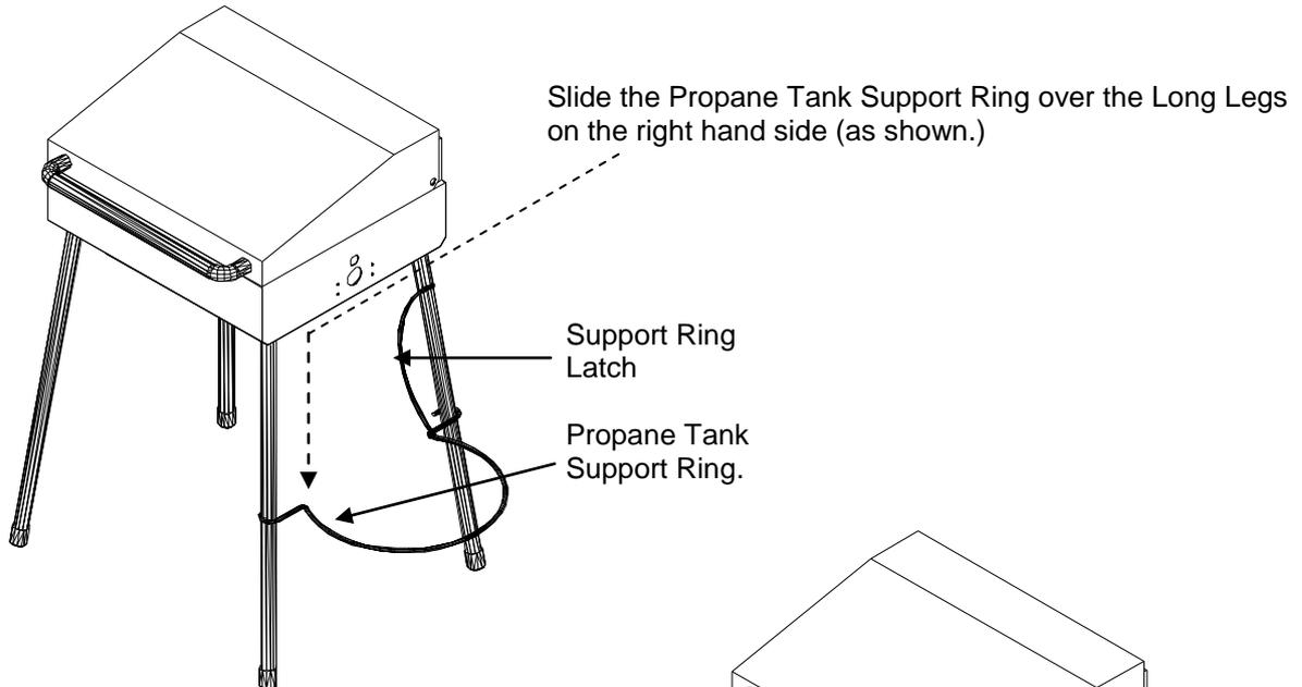
Place the Propane tank inside the tank ring (as shown.)
