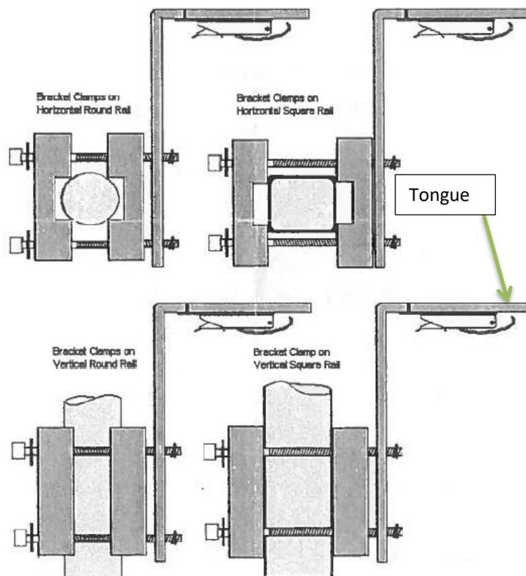
Figure 3: Rail Mount (Horizontal and Vertical Mount)
