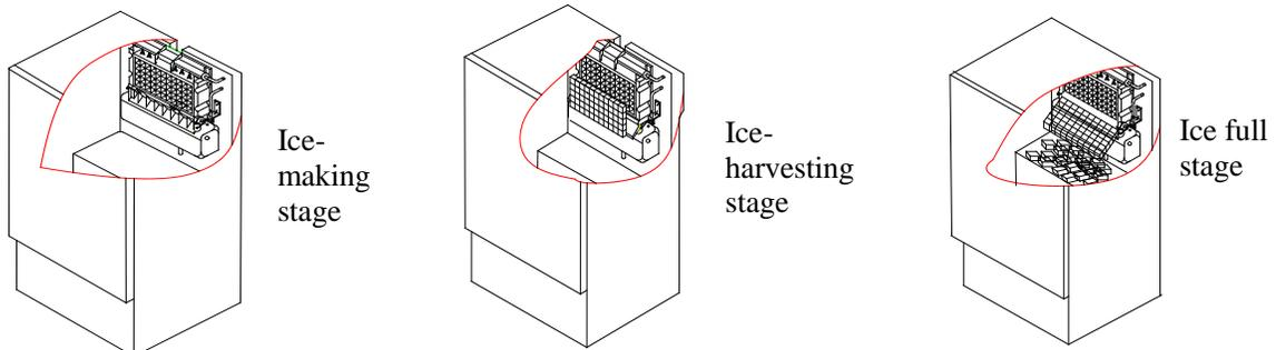
2. After three minutes, the machine will automatically go into the ice-making stage, and the sound of flowing water will be heard.
