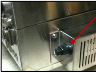
Fig. 3: Regulator Valve Lighting Position
